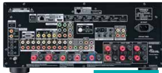
Painel traseiro do Receiver DTR 50.7
